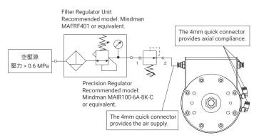
2. Check the center point (\*1) of the compliance module. Apply 0.2 MPa air pressure while the module is stationary. Verify the air supply connectors: one extends the LCZA300, the other retracts it. Confirm the correct direction before use. Ensure the compliance module returns to the center point, as shown in the illustration below. If it does not return to the center point or is misaligned, contact your supplier.
