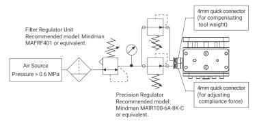
2. Check the CENTER POINT (\*1) first; giving 0.2 MPa pressure to the compliant force connector while the spindle is turning off. Make sure the spindle is able to return to the CENTER POINT as shown as the illustration below. Please contact your supplier if it couldn't return to or is not on the CENTER POINT.
